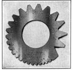
FIG. 141. N. F. Thread Gauge.
