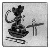
FIG. 227 Valve Stem and Cutter Grinding Attachment.
