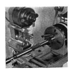
FIG. 232A Grinding Solid Reamer.
