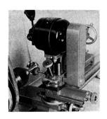
FIG. 226 Grinding 90° Valve.
