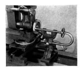
FIG. 230. Grinding Valve Stem.
