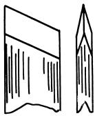
FIG. 274 Large Skew Chisel.
