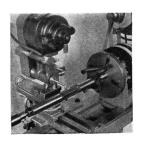
FIG. 232A Grinding Solid Reamer.
