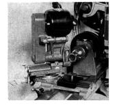
FIG. 225. Grinding 45° Valve.
