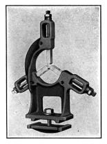
FIG. 180 Steady Rest, or Center Rest.
