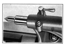
one on each end of the gib, regulate the tightness of the tailstock between the bed ways. These two screws should be adjusted evenly so that both ends of the gib will bear against the way with the same amount of pressure.
